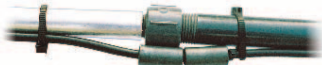
Figure 5 — Ferrite bead common mode choke at base of driven element.
