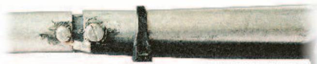
Figure 4 — View of driven element coax cable attachment.
